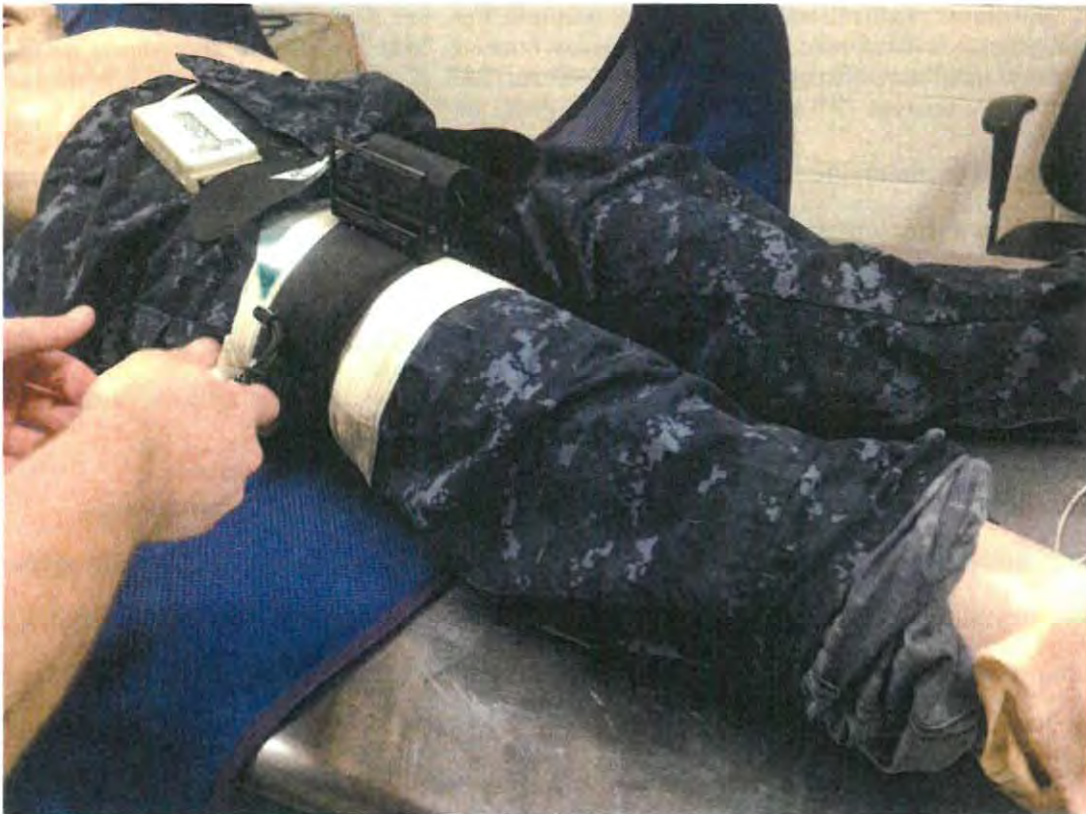
Figure 12. Example tourniquet application to the SSH. The Tekscan pressure sensor was secured to the thigh of the SSH with an elastic bandage and the EMT is applied over it. The patient sling was beneath the SSH during the application, ready for the simulated transfer after five minutes of occlusion.
