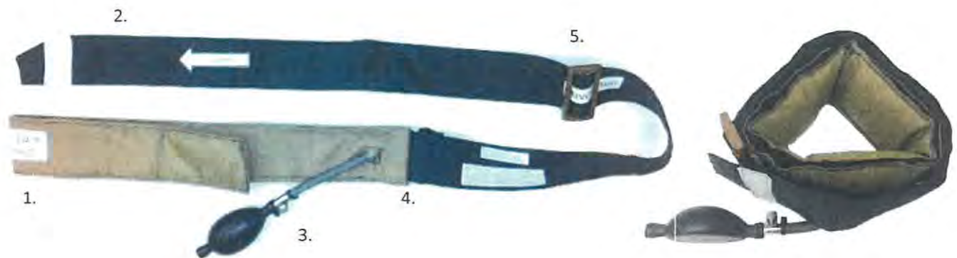
Figure 8. Tactical Pneumatic Tourniquet. 1. Inner layer of strap material (tan) with integrated air bladder and hook-and-loop fastener. 2. Outer layer of strap material (black) with integrated hook-and-loop fastener. 3. Hand bulb pump. 4. Hook portion of clasp for outer strap. 5. Clasp with outer strap threaded through slip lock mechanism.
