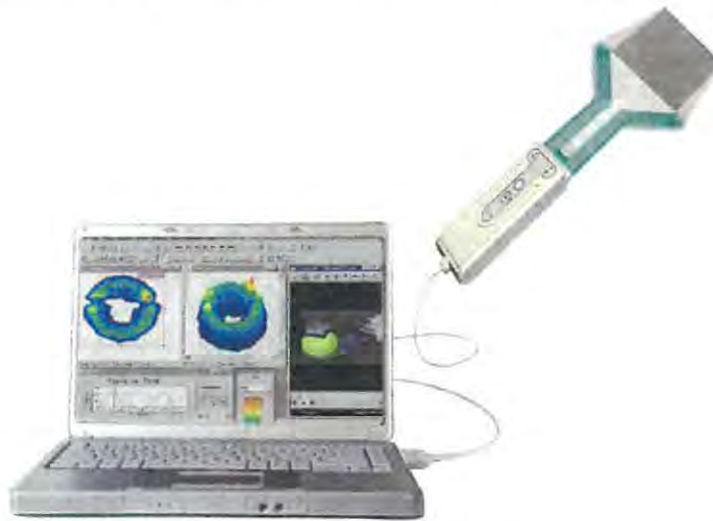
Figure 2. Tekscan I-Scan ® Pressure Measurement System. The Tekscan pressure measurement system senses and maps pressure distributions across its sensing surface. The scanning electronics rapidly record data from an array of independent sensing elements contained within each sensor.
